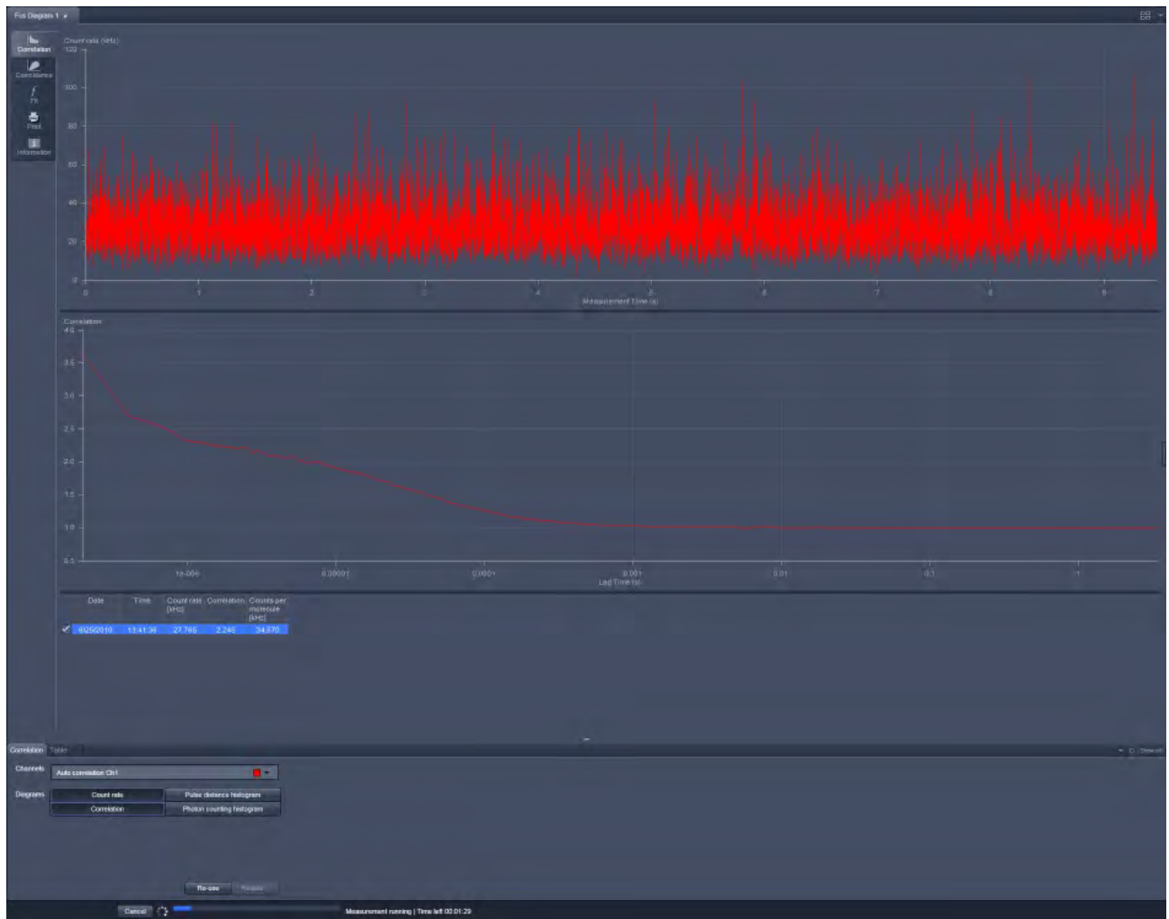
Fig. 351 FCS Correlation window during data acquisition
