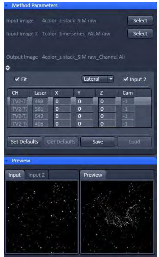
Fig. 512 Two images mismatched in their dimensions (Z-Stack SIM raw and time-series PALM) images loaded
