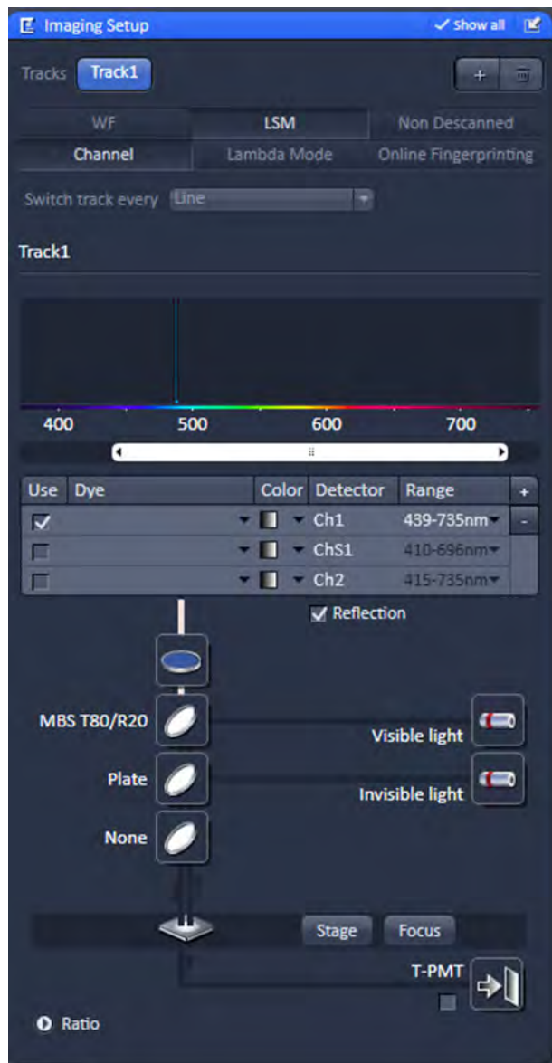
Fig. 305 Beam path configuration for finding glass reflection
