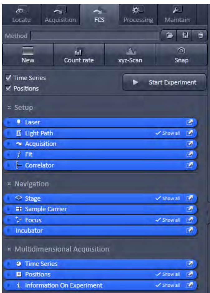
Fig. 258 FCS tool group (Note that Time Series and Positions tabs are only available, when the corresponding boxes have been checked)
