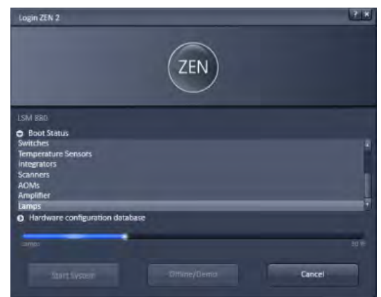
Fig. 10 Starting the ZEN software – The Login "ZEN" dialog with Boot Status field expanded and during the process of booting
