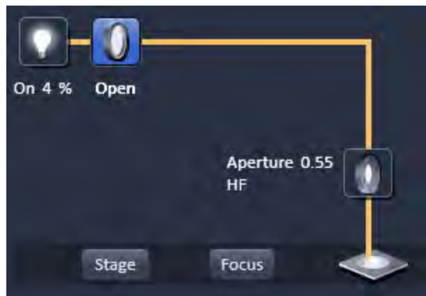
Fig. 49 Microscope Control tool – HAL lamp switched on, shutter in the Open position
