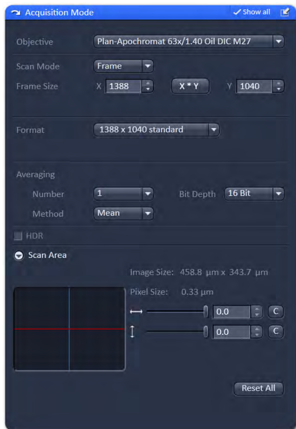
Fig. 137 Acquisition Mode - Frame with Camera tab selected in the Imaging Setup tool
