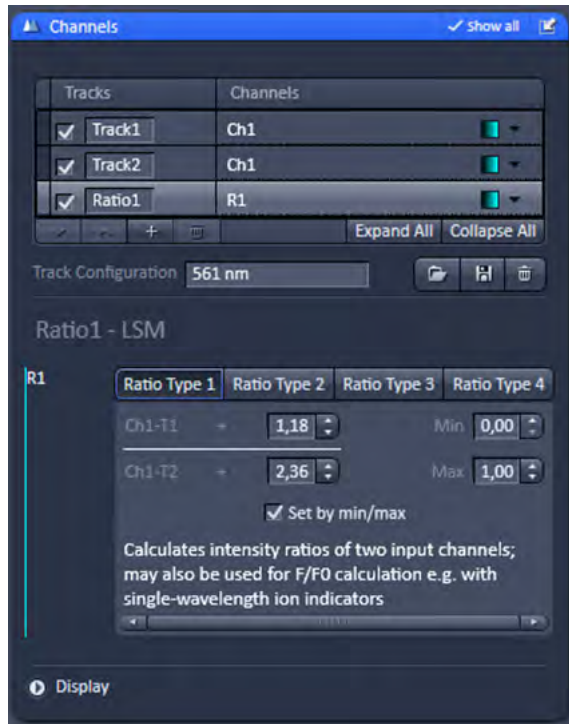
Fig. 749 Channels tool with Ratio Type 1 formula selected for the Ratio1 channel using a G factor of 1.18
