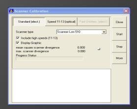
If the small dot in the middle of the window is grey or green, the calibration was successful and you can close the window.
