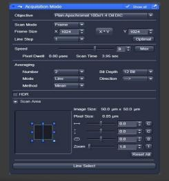
In the Acquisition Mode window set the Frame mode, Frame Size of 1024x1024 pixels, Line Step of 1.
