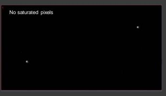
The **Digital Offset** must be set above zero (~12) so that no pixels read zero intensities.
