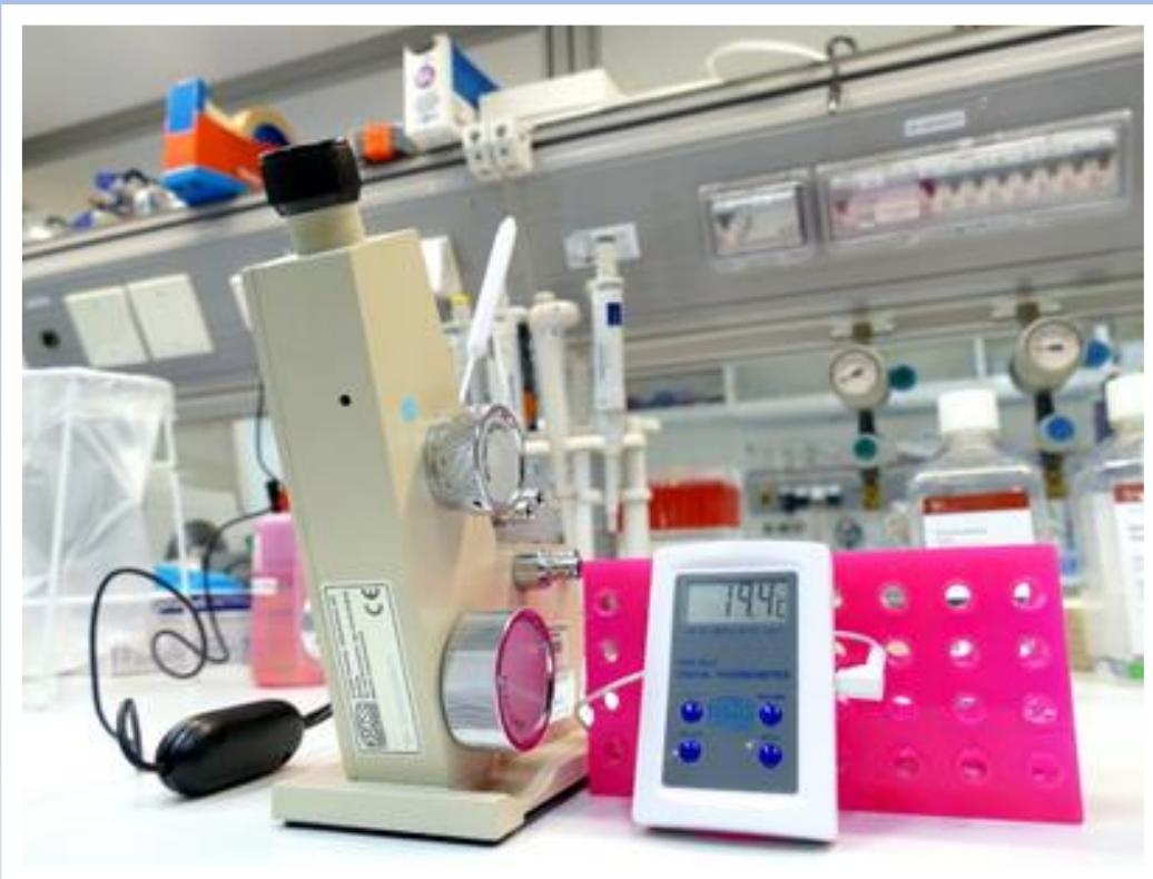
**Refractometer for refractive index measurements**
