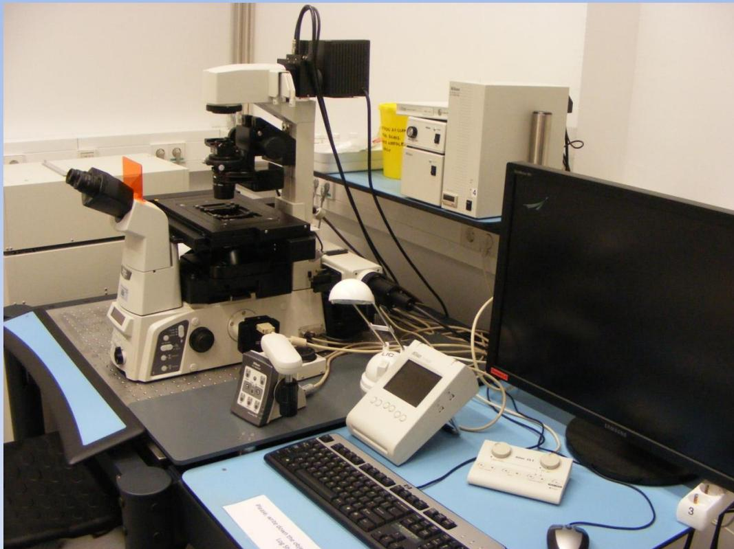
**3-channel + spectral detector confocal microscope with**
