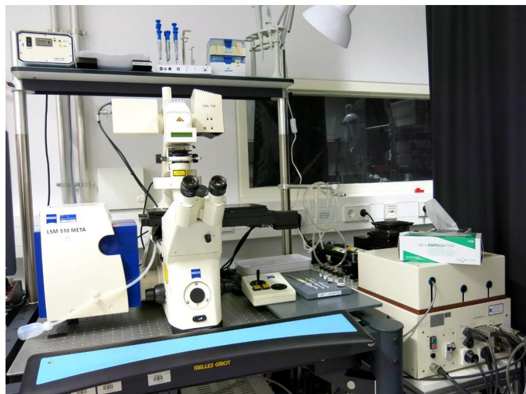
**3-channel confocal microscope with**
